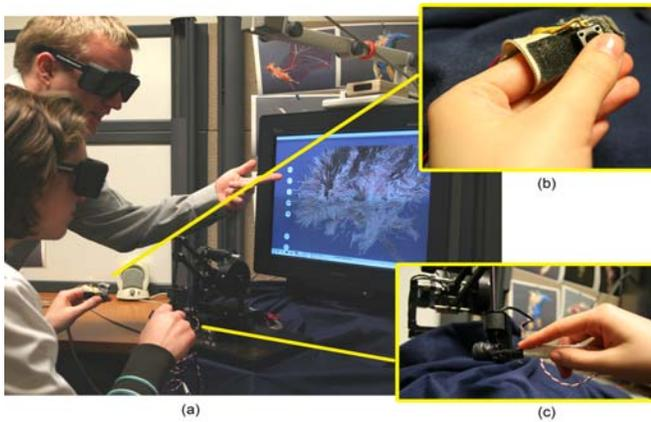
Figure 2: Users collaborating on hypotheses about WM connectivity using 3D lasso drawing selection interface in 3D stereo VR. (a) Fishtank VR setup. (b) 3D hand tracker. (c) Phantom force feedback device.
