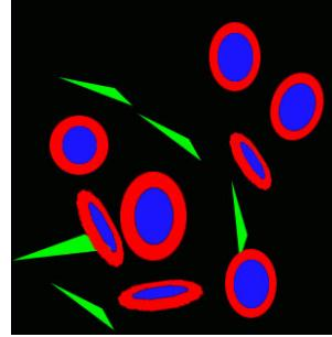
**Figure 1c:** Pre-Visualization Image. Glyphs represent velocity, magnitude and vorticity.
