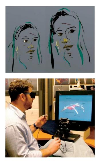
But how the images above have been produced? "Drawing on Air uses a stereoscopic desktop display. A Phantom haptic device and 6-Degree-Of-Freedom (DOF) trackers are used for a two-handed input." (Credit: Brown University)
