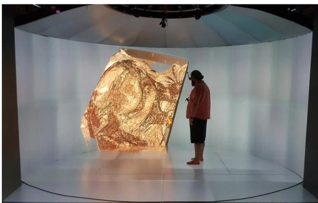
Figure 3. The Brown University YURT with a user inside. The OptiTrack cameras line the ring and the straight edges of the ceiling.
