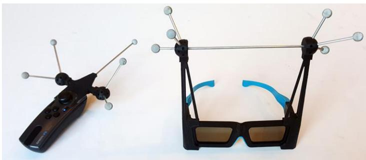
Figure 4. The wand and glasses used in the YURT. Attached to each tool is a constellation of reflective balls used by the optical tracking system to compute its location. The glasses use active shutters with 120Hz frequency to let users see stereo 3D.
