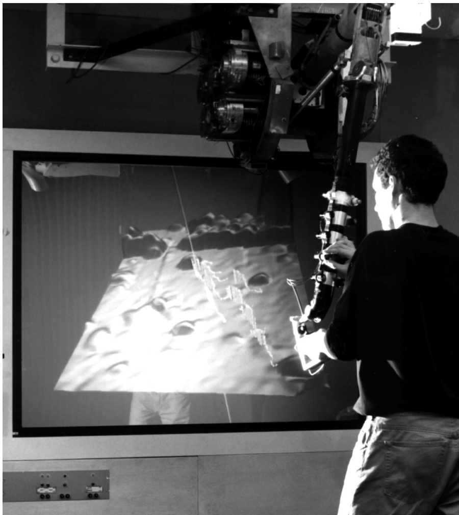
Figure 3. Using an atomic force microscope, Michael Falvo taps a gold ball into the desired gap in a circuit. (The entire field of his view is 1 nm.)
