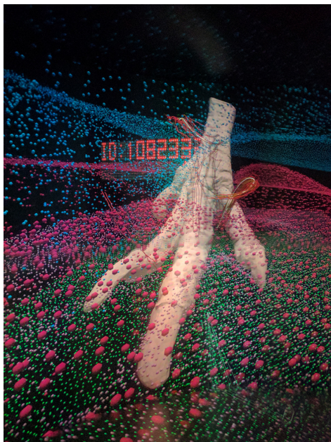
Fig. 2: Example visualization of particle flow during dinosaur track creation. To avoid visual clutter we only show four thin layers of simulated particles, color coded based on their initial depth (from blue on top over red and magenta to green on the bottom). A tooltip display indicating selected particle ID's can be seen in the background.
