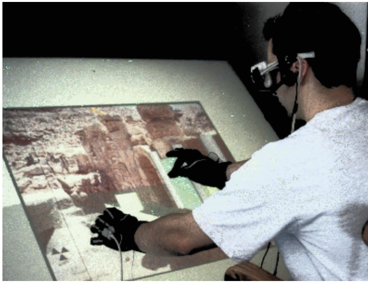
Figure 5: Illustration of a gestural and voice-driven user interface for interactively modeling 3D objects in a virtual environment. Simple geometric models here are overlaid on a photograph from the site at Petra. Stereo shutter glasses show each eye a different image, a microphone picks up speech, and gloves detect gestures and hand location, permitting natural 3D object manipulations. The large-sized screen is a BARCO Baron projection table providing a semi-immersive environment.
