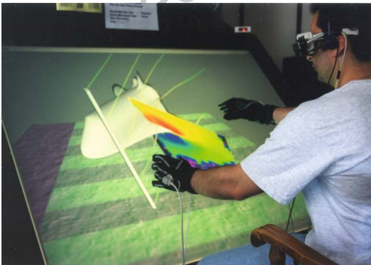
Fig. 10.2 A user interacting with a dataset for visualizing a flow field around a space shuttle. The user simultaneously manipulates the streamlines with his left hand and the shuttle with his right hand while viewing the data in stereo. The user asked for these tools using speech input
