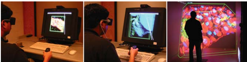
Fig. 10.10 Experimental setup for the exploring scientific datasets. Scientists examine a range of datasets on a conventional desktop (left), Fishtank (middle), and Cave (right) environment. (Note: different datasets are shown on each display in these images.)
