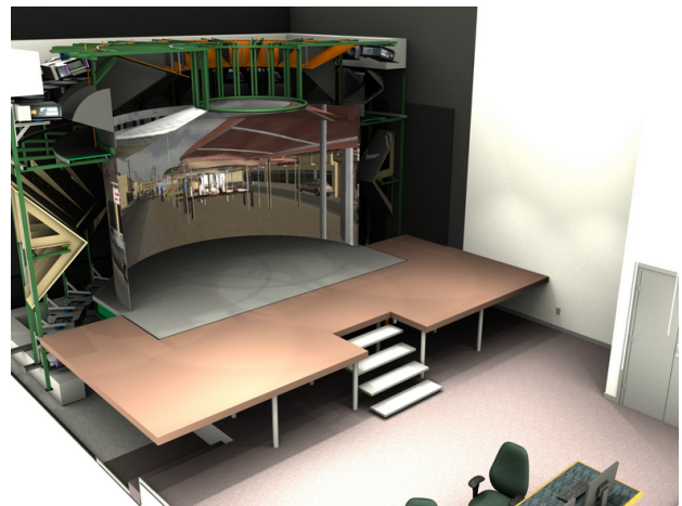
Figure 1: Artist's rendering of the new Cave based on CAD drawings (The front part of the screen, the doors, is omitted in this image).
