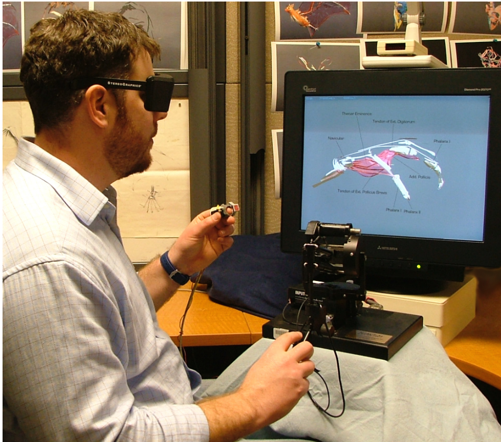
Figure 3.2: Drawing on Air uses a stereoscopic desktop display. A Phantom haptic device and 6-DOF trackers are used for two-handed input.
