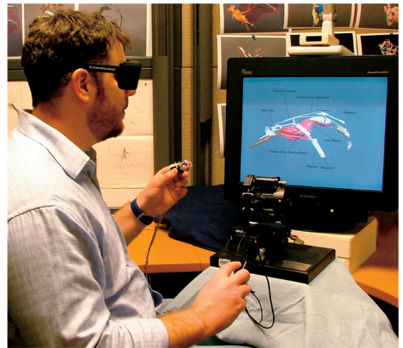
Fig. 2. Drawing on Air uses a stereoscopic desktop display. A Phantom haptic device and 6-Degree-Of-Freedom (DOF) trackers are used for a two-handed input.
