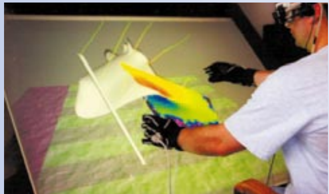
F A user interacting with a scientific data set. He uses a multi-modal interface combining hand gesture and speech to change modes and application state, such as creating and controlling visualization widgets, and starting and stopping recorded animations.
