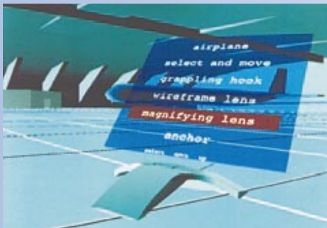
G The display geometry of the virtual tricorder closely reflects the geometry of the 6DOF Logitech FlyMouse, enhanced with transparent menus.
