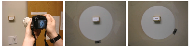
Figure 1: Manual focus with vision-based interaction. As the photographer rotates a cardboard barrel around the lens, the dark marker inside is positioned around a reserved region of the image, and the focal length changes from shallow to deep. Sample video of this feature is available at: http://www.cs.brown.edu/people/steveg/camvids.html .
