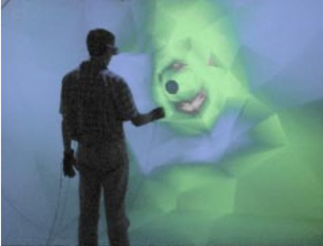
Figure 4: Wall shear stress is encoded in wall color (see color plate), with blue showing low values, green midrange values, and red high values. Regions of low shear stress tend to be correlated with sites of future lesions.
