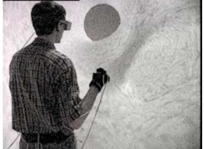
Figure 3: A view of the immersive artery visualization looking at the bifurcation where the graft enters the original artery. The visualization is within a 4-wall Cave (3 walls and a floor), with head-tracked stereo. A gestural interface provide easily-learned interaction techniques for navigating through the environment and for studying the flow.
