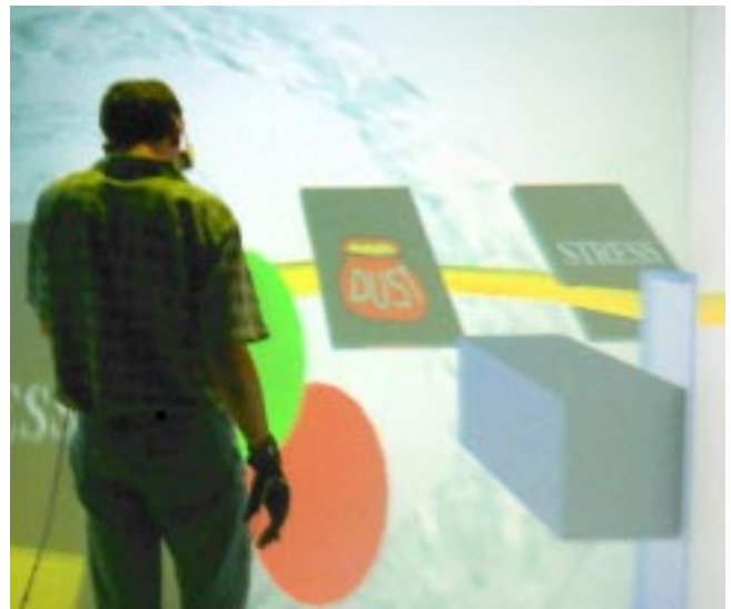
Figure 6: When the user looks down a toolbelt appears. Tools include dust, for advecting particles through the flow; a widget for choosing wall coloring; a round alkaseltzer widget for creating a persistent source of advecting particles; an isosurface “microphone” widget (the square cube here); and a streamline and rake widget.
