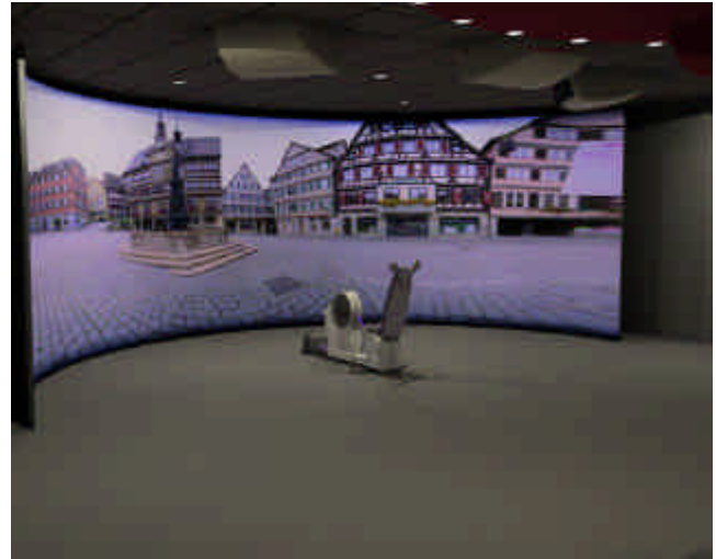
Figure 2: Virtual reality setup. 180°, 7m diameter VR theatre with recumbent bicycle positioned in the centre displaying "Virtual Tübingen".
