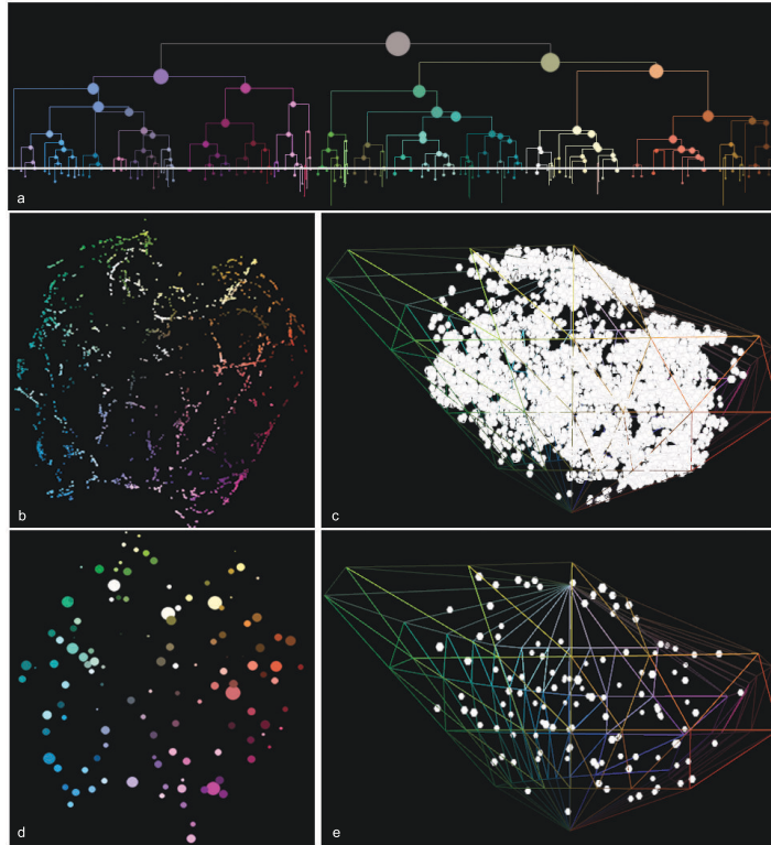
Fig. 6: A clustering cut in the dendrogram view (top row) is applied to the linked 2D embedding and 3D colorer (middle row). Points belonging to the same cluster are collapsed to their centroids (bottom row).
