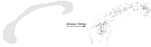
Figure 4: Seed points are adjusted so that Euclidean distances between the points on the plane reflect the distances between their associated integral curves.
