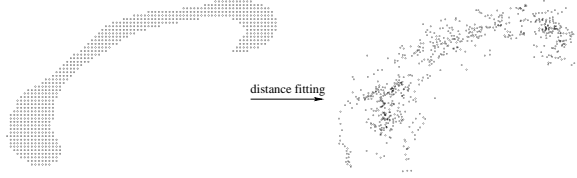
Figure 4: Seed points are adjusted so that Euclidian distances between the points on the plane reflect the distances between their associated integral curves.
