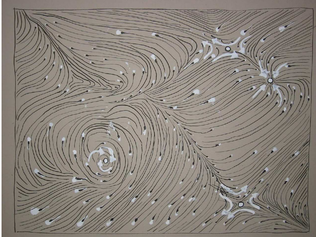
Figure 4.7: After the experiment, designers were asked to create a new visualization design that would outperform the six methods presented. This image shows one of the results. Black flow lines help in the advection task, and white marks indicate direction of the flow. Critical points are clearly marked by large white dots, and critical point type is indicated by the surrounding arrows.
