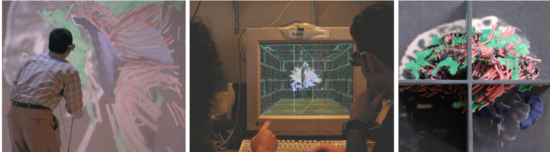
Figure 2.8: Three different visualizations of the diffusion tensor magnetic resonance imaging data of a brain. This tensor field data can be explored using an immersive VR environment such as a CAVE (left) [Zhang et al., 2003], a fish-tank-VR setup (center) [Demiralp et al., 2006], or a physical model created through color rapid prototyping (right) [Acevedo et al., 2004].
