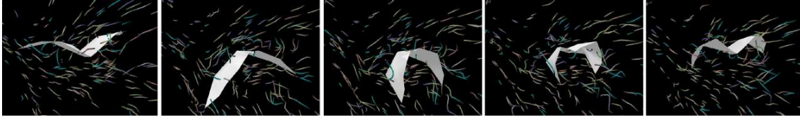
Figure 2.7: Particle flurries in a Virtual Reality visualization of air flow around a bat in flight [Sobel et al., 2004]. Over a short time, the particle animation gives a synoptic visualization of the main features of the three dimensional vector field.
